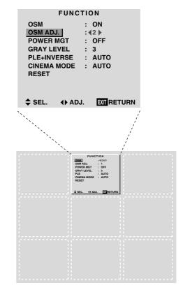
Once all adjustments are completed ... Press the "EXIT" button to return to the main menu. To delete the main menu, press the "EXIT" button once more.
